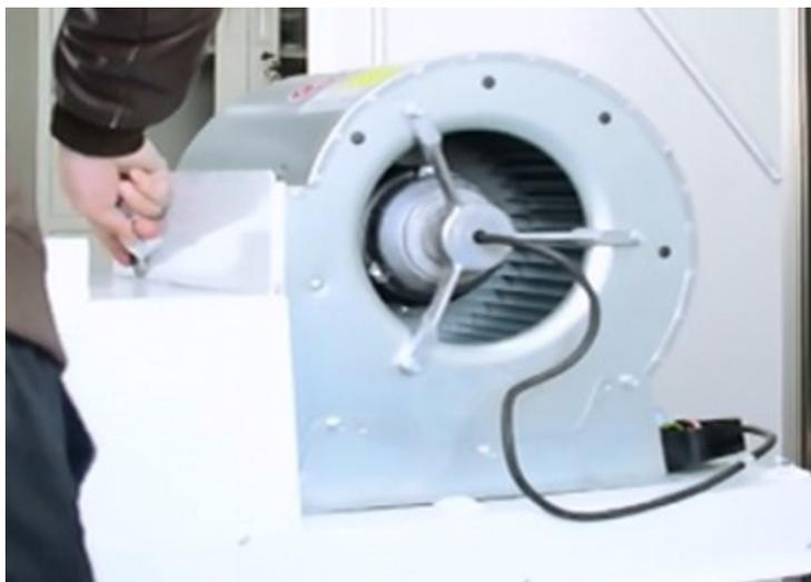
M) Remove the fan and mounting plate connecting piece
