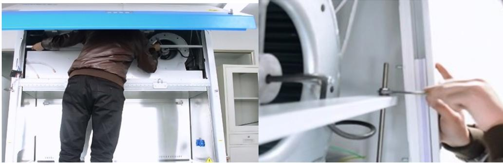
w) Install the front panel and travel switch bracket.
