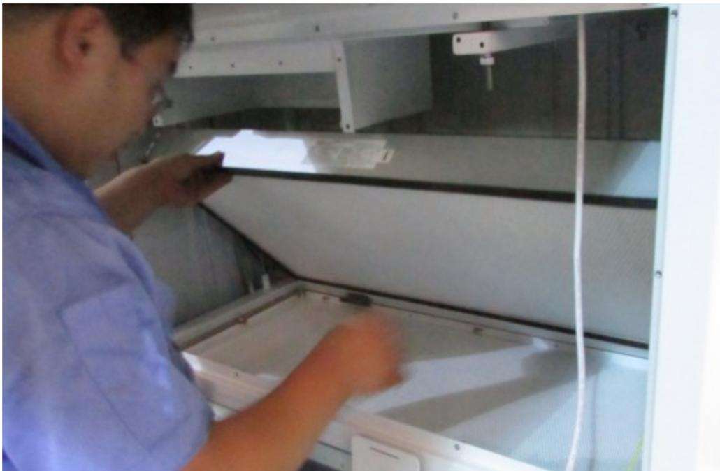
i) Remove upper press bar, remove the upper filter and plate
