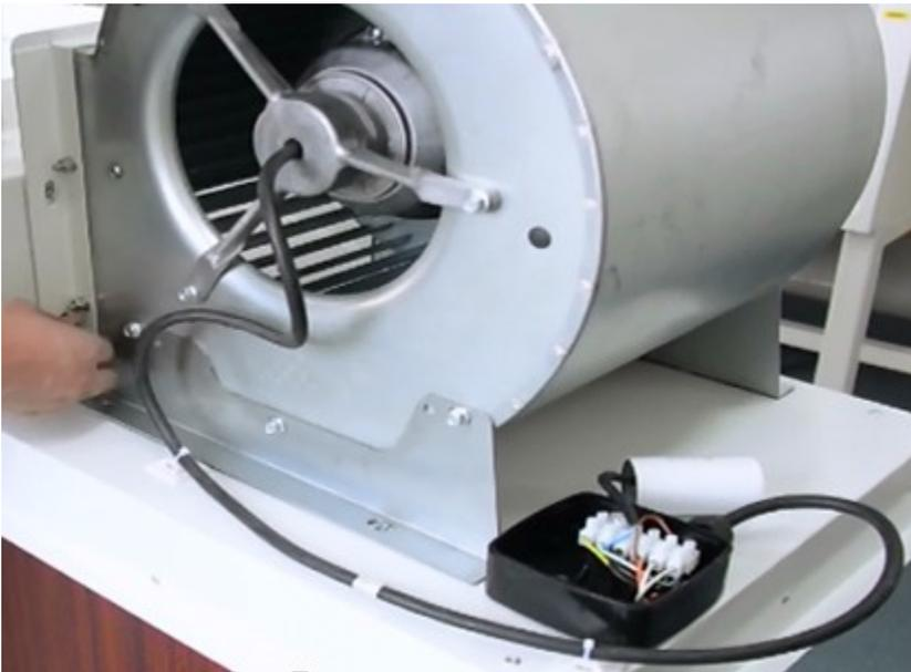
l) Cut white porcelain between the fan and fan plate with a blade.
