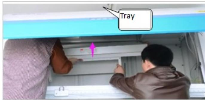
j) Replace the same type of upper filter, adjusting tray and filter, reconnect ducts, tighten screw nuts
