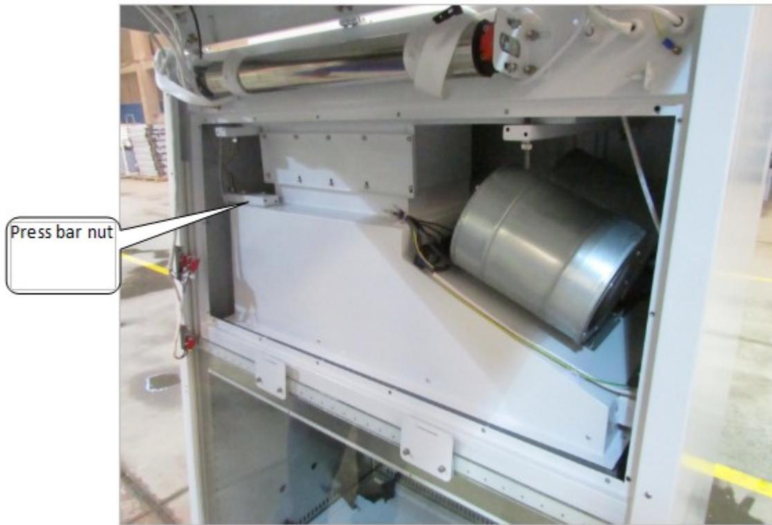
d) Remove air duct connecting plate
